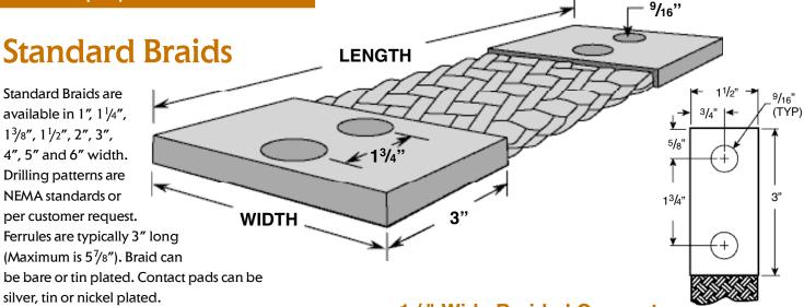
Current capacity to 3200 amps is available. Current capacity is based on a single conductor in free air with a temperature rise of 30 degrees centigrade, or 50 degrees centigrade.
